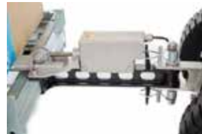
Electrical locking module for hook
